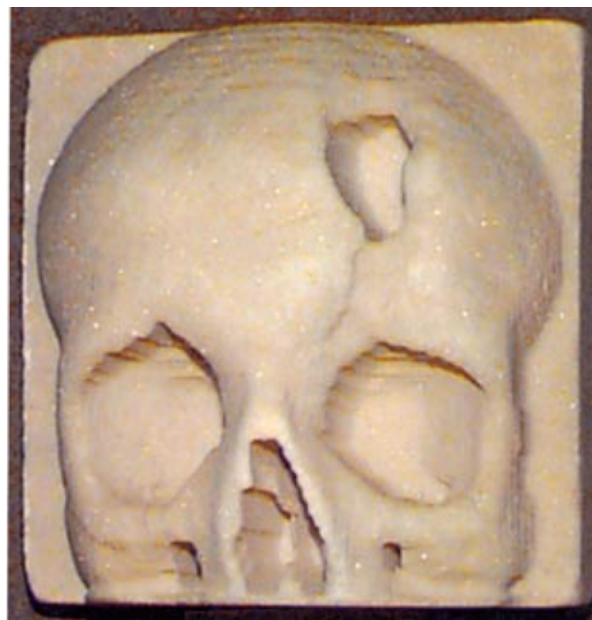
Fig. 5. The surgical model made by using computer derived surface co-ordinates from the data visualised in Fig. 2 to drive a numerically controlled milling machine.
